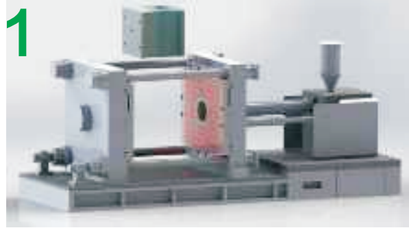
1 注塑机开模，吊入模具 The injection molding machine opens the clamp platen, and lifts the mold into the machine.
