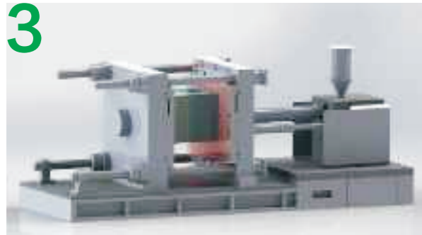
3 注塑机合模，并高压锁模，转动安全钥匙的同时按下定模、动模充磁按钮 The injection molding machine closes the mold, and clamps the mold with high pressure, and presses the fixed mold magnetizing button and movable mold magnetizing button while turning the security key.
